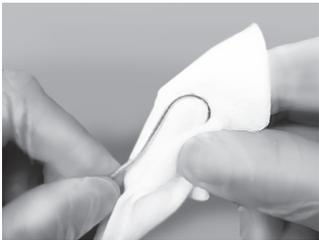
Wipe the file holder, long file holder and contrary electrode with a piece of gauze dampened with Ethanol for Disinfection (Ethanol 70 to 80 vol%).
