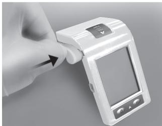
1. Insert the probe cord completely into the jack on the left side of the S-Apex.
