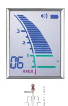
The meter is activated when the file is inserted into a root canal. The number of bars remaining before the file reaches the flash bar is shown in the lower left corner of the display. When the file tip reaches a position near the apex, the bar color changes to green to indicate you have reached a critical area.
